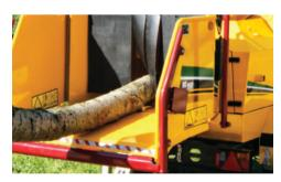
MARKET-LEADING INFEED. An exceptional 20 x 30.5 cm infeed opening fed by oversized horizontal offset feed rollers and auto reversing SmartFeed control provides the capacity and power to do the hard work for you.
