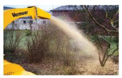
NO-COMPROMISE CHIPPING. Coupling the Kubota 48,1 hp (35,9 kW) engine to a 76 cm diameter 4-knife disc, the BC190xL deals with diameters up to 20 cm and throws it at an average distance from 10 to 12 meters, yet all this at 120 dB(a)!
