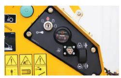
**PUSH-BUTTON CHIPPING.** Automatic cutter disc start at the push of a button helps provide convenient operation and allow engine starting without load for enhanced reliability.
